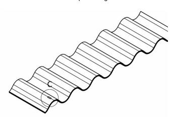
corresponding the purlins of the supporting structure and the thermal expansion of polycarbonate panels.
